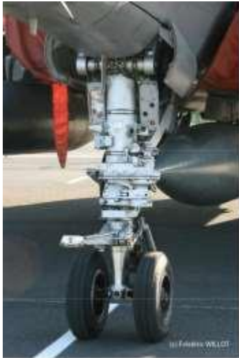
Twin wheels Nose gear of a Rafale
