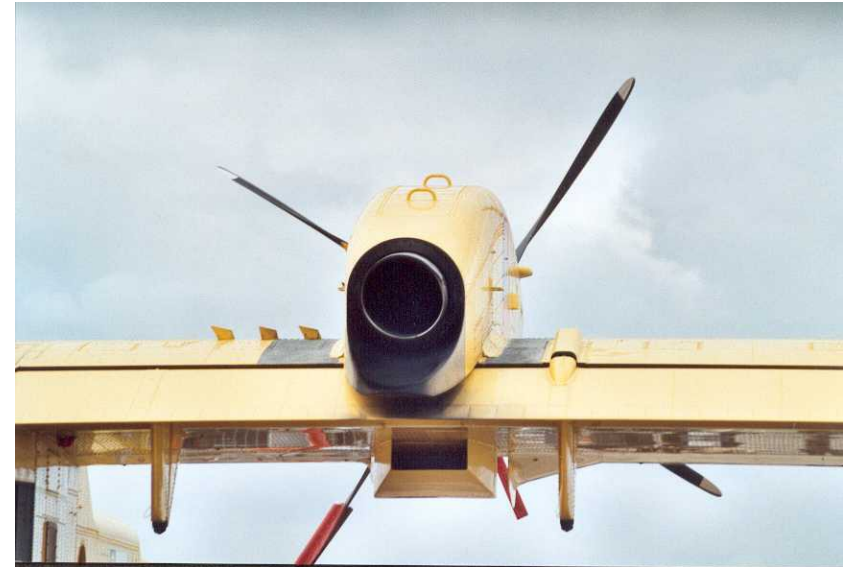
Overwing nacelle mounted engines
