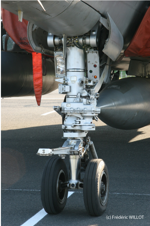
Twin wheels nose gear of a Rafale
