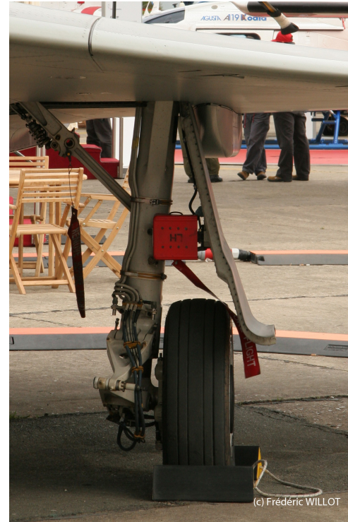
Single wheel main gear of a Typhoon
