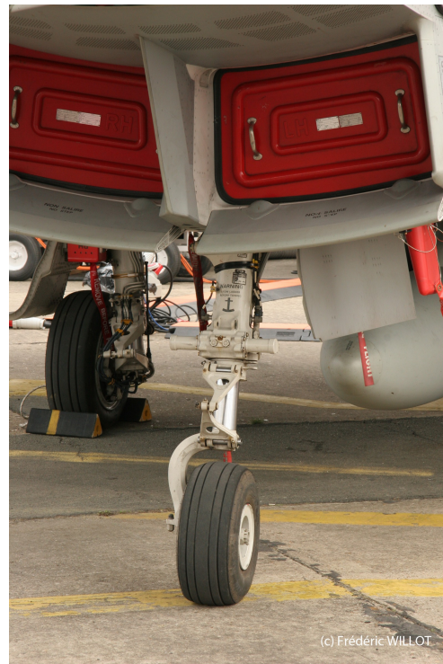
Single wheel nose gear of a Typhoon
